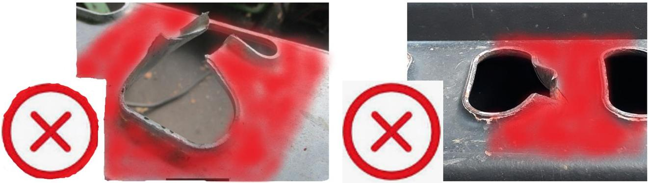
Fig 5. Cracked hook passage holes prohibited for lashing
