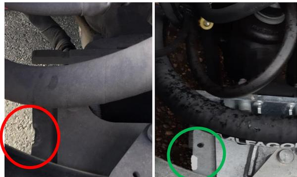
Fig 1B: Drawbar: contact imprint - repaired repainted
