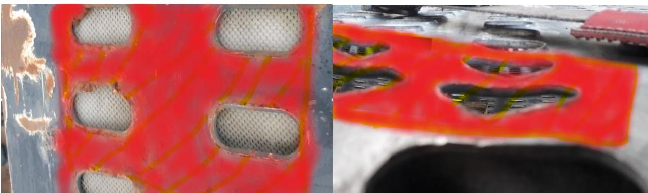
Fig. 4. Surfaces prohibited for supporting a strapped wheel
