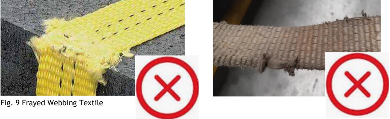
Fig. 9 Frayed Webbing Textile
