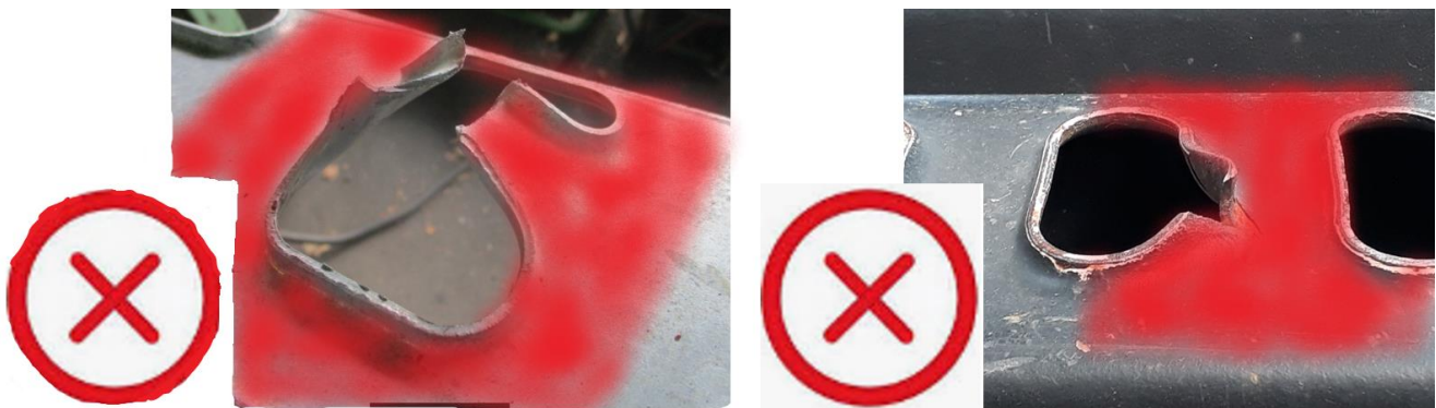
Fig 5. Cracked Hook Passage Holes Prohibited for Securing
